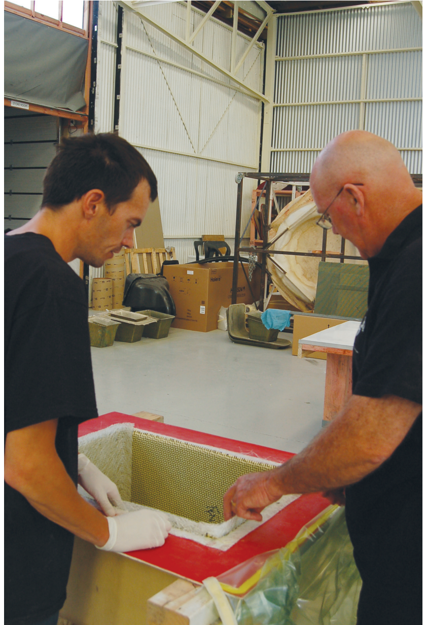
Scott Nicholls and Peter Maloney attending to a fuel tank mould setup
